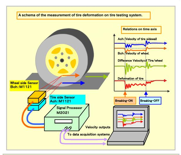
The figure pictured above is a diagram of the measurement of tire deformation for automobile under hard breaking by using 2-channel Laser Doppler Velocity Meter MODEL-2021.
