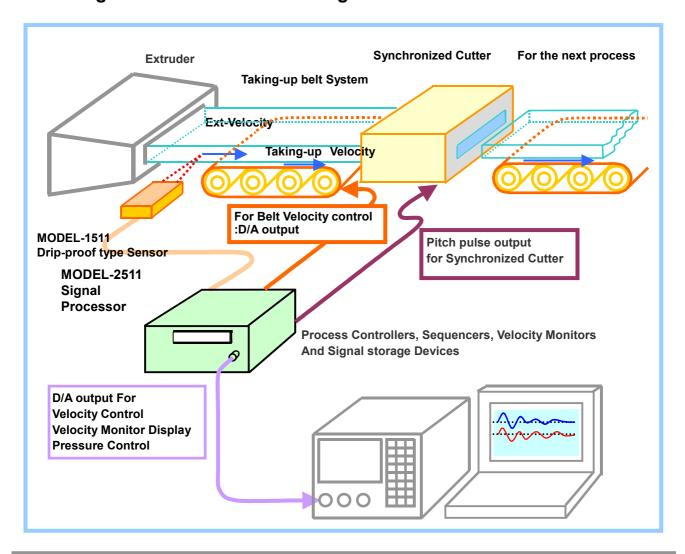
**MODEL-2511** is a Laser Doppler Velocity meter that is appropriate for the control field where the **drip-proof type sensor** is assumed to be a feature under the **Non-Contact** condition.
