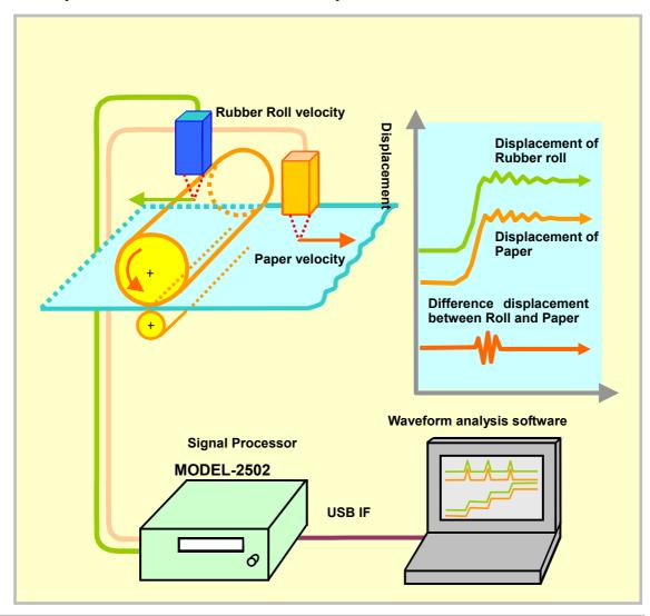
The application shows **MODEL-2502** is used in developing **the copy machine or the printer**. MODEL-2502 can measure **"Irregularity of the amount of paper feeding"** by the behavior of **"Slipping"** generated between the paper feeding rubber-roller and the paper directly because it has the **calculation function between two channels**.
