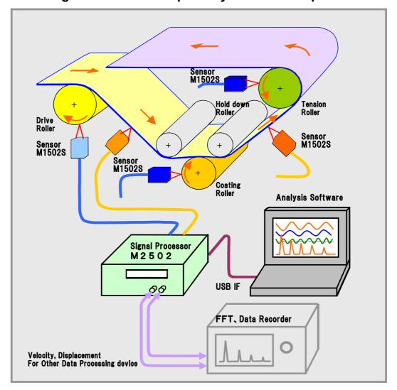
The figure pictured above is a diagram of the coating process on the transparency film for LCD panel, by using 2-channel Laser Doppler Velocity Meter MODEL-2502.
