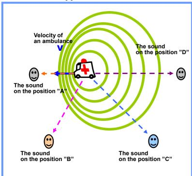
The Doppler effect means the phenomenon in which the wavelength (frequency) of the wave which a watcher measures differs compared with it in a generation source, when the velocity difference relative between the generation source of a wave (sound, light, and electric wave) and a watcher has arisen.
